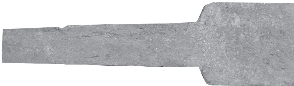
Figure 37: Surface of iron after forging
