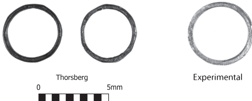
Figure 88: Two rings from Thorsberg showing facets on the outside diameter
