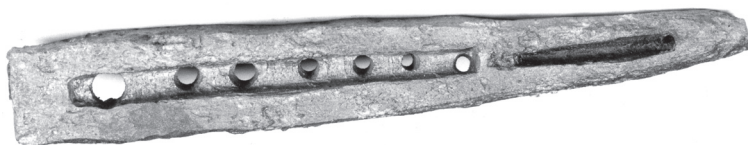
Figure 77: Cast of a draw plate from Altena (207mm long, 31.5mm wide and 17mm thick)
