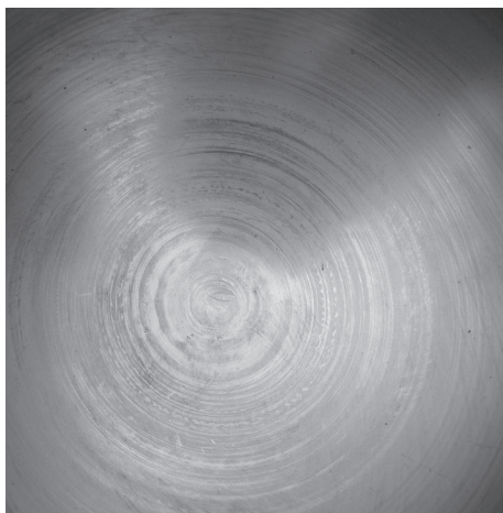
Figure 38: Spinning marks on a reproduction helmet
