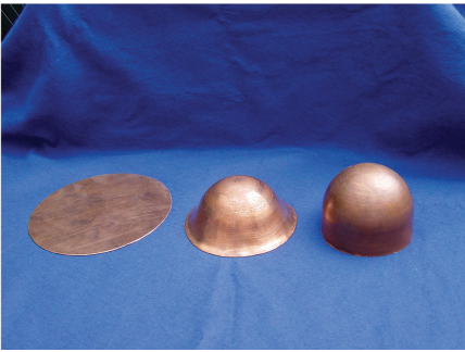
Plate 2: The spinning process in a contemporary workshop.
